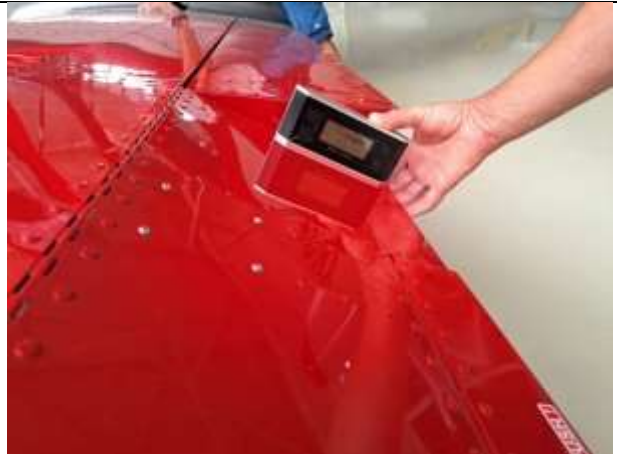
Fig. 6-12 Measure and record left aileron down deflection
