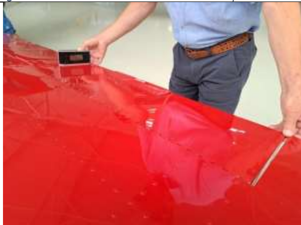
Fig. 6-8 Set aileron to neutral position against wing tip and place digital protractor on the aileron root and zero it.
