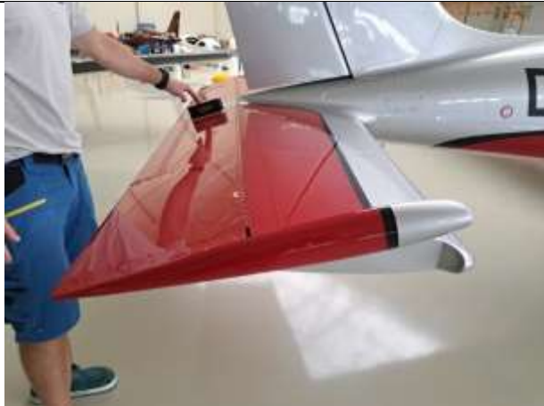
Fig. 6-18 Measure and record elevator down deflection
