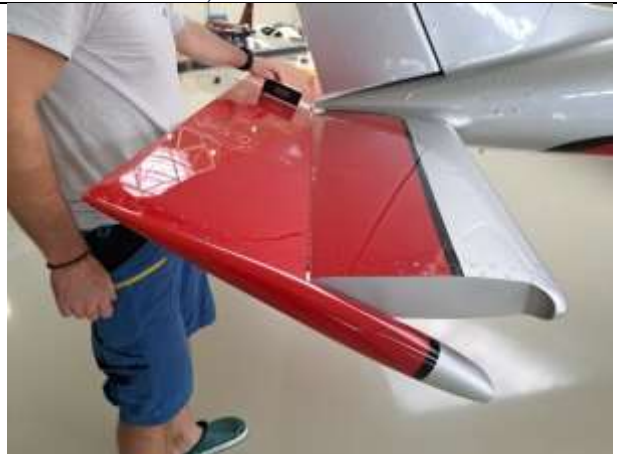
Fig. 6-16 Measure and record elevator up deflection
