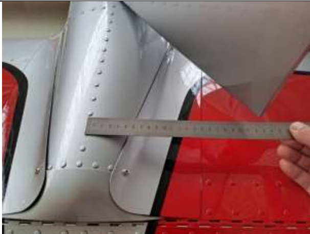
Fig. 6-19 Rudder right deflection. 30° = 225 mm
