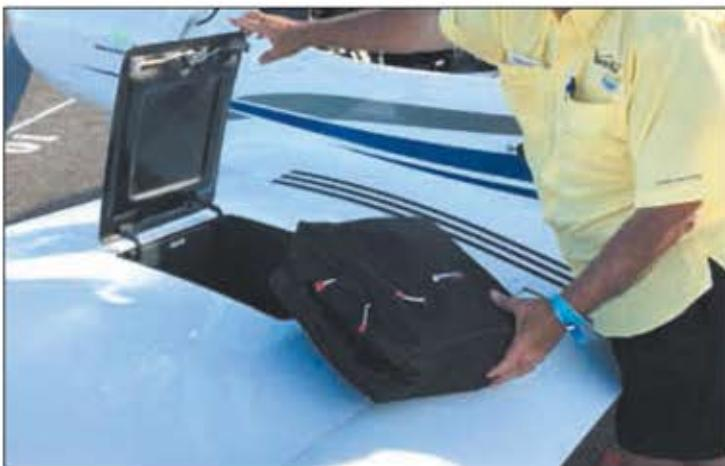
*Landing gear, left, is an LSA weak point. Bristell claims to have reinforced its gear and the nosegear is steerable. Each wing, lower photo, has a unique baggage locker with a 44-pound capacity.*
